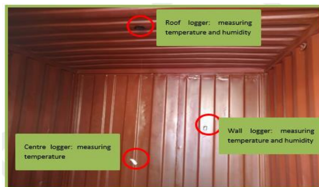
Figure 9: Configuration of logger placement in the container
